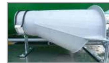
Flowing concrete chute
